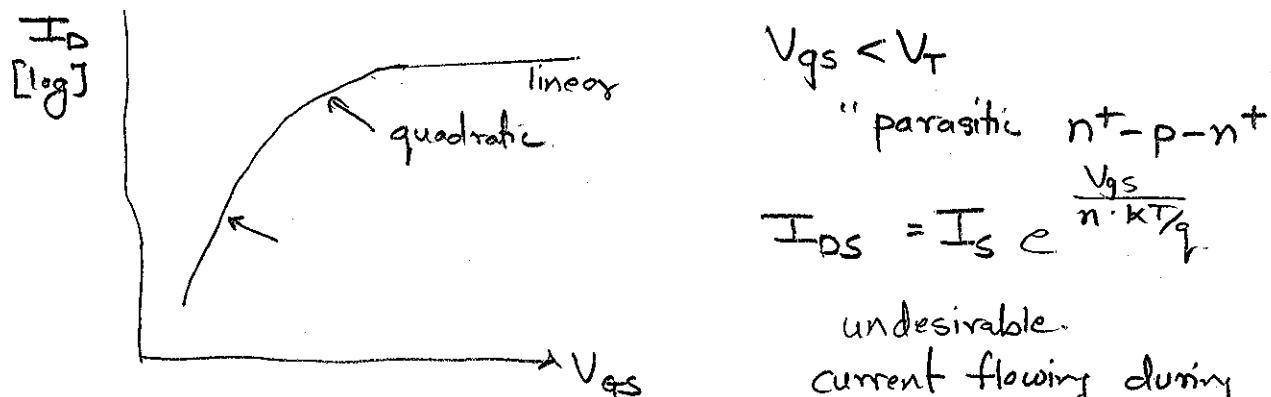
(inverse) rate of decline of current wrt.  $V_{gs}$  below  $V_T \rightarrow$  quality of device
